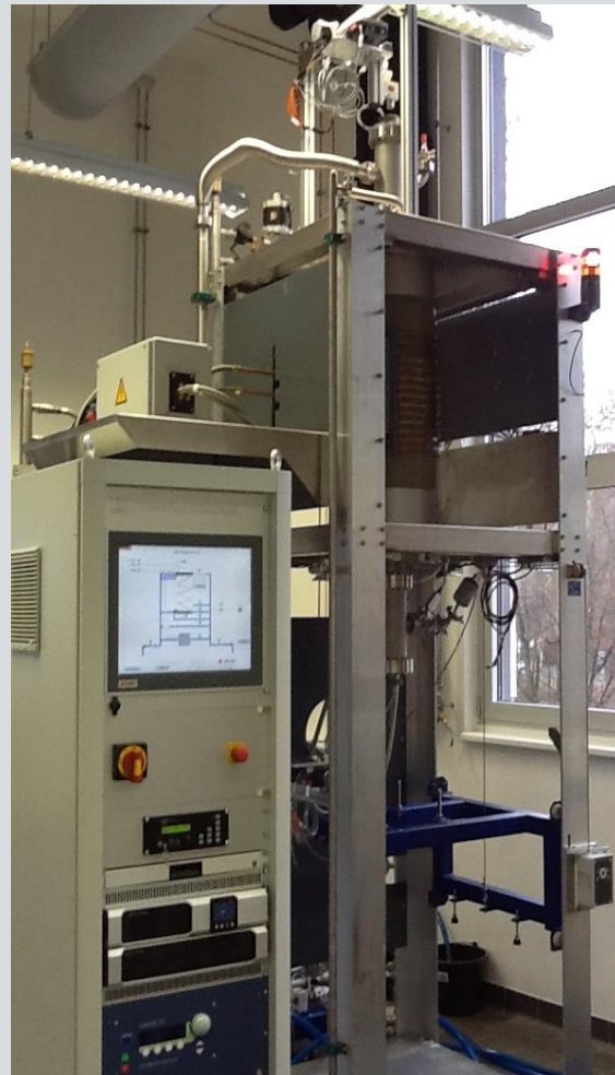
4inch SiC PVT reactor designed & manufactured at the machine shop of FAU
